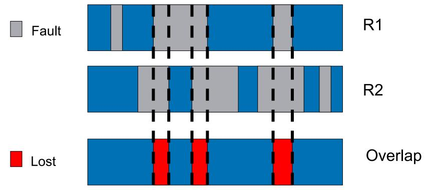
•Faults may be bits, sectors, files, disks, arrays, etc.
