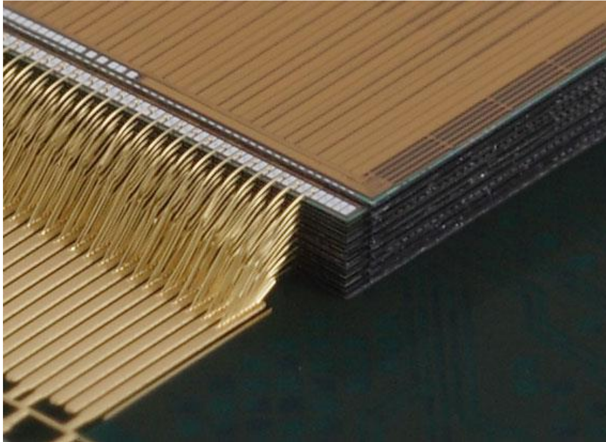
Akita Elpida wire bond example of 20 stacked die(40u pitch)
